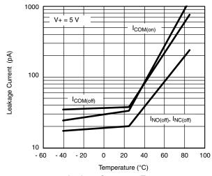
Leakage Current vs. Temperature
