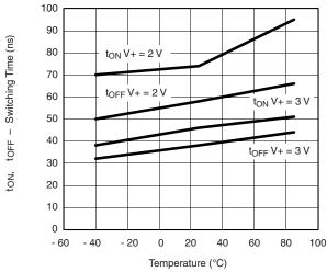
Switching Time vs. Temperature and Supply Voltage
