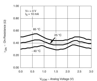
r<sub>ON</sub> vs. Analog Voltage and Temperature
