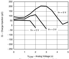
Charge Injection vs. Analog Voltage
