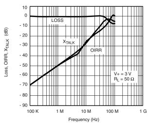
Insertion Loss, Off-Isolation, Crosstalk vs. Frequency
