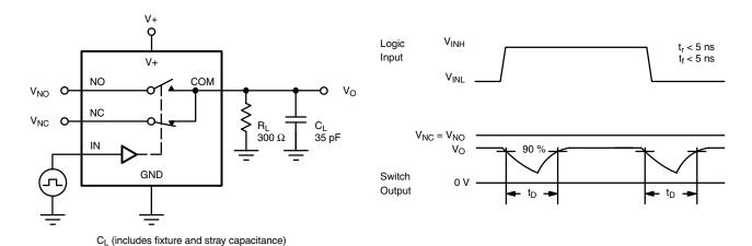
Figure 2. Break-Before-Make Interval
