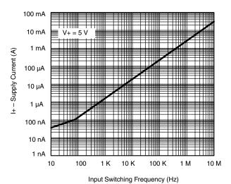
**Supply Current vs. Input Switching Frequency**
