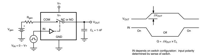
Figure 3. Charge Injection
