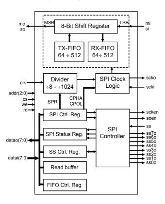
**Receiver FIFO** - The Rx FIFO can be 64 (128, 256, 512) levels deep, it receives data until the number of bytes in the FIFO equals the selected interrupt trigger level. At that time if interrupt is enabled, the DSPI FIFO will
