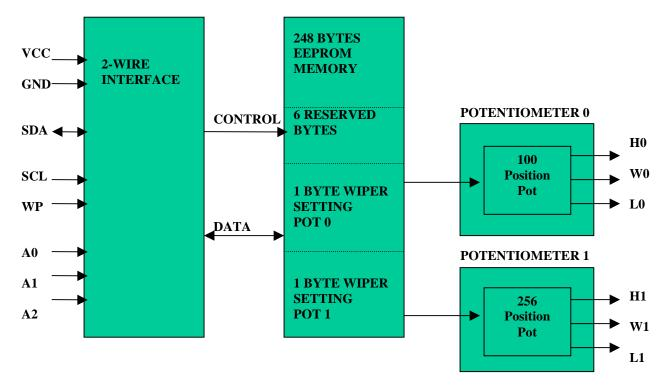
Up to eight DS1845s can be installed on a single 2-wire bus. Access to an individual device is achieved by using a device address that is determined by the logic levels of address pins A0 though A2. Additionally, the DS1845 will operate from 3 volt or 5 volt supplies. Three package options are available: Flip Chip Package, 16-ball STPBGA and 14-pin TSSOP.
