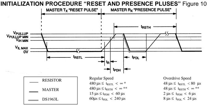
\*IN ORDER NOT TO MASK INTERRUPT SIGNALS BY OTHER DEVICES ON THE 1-WIRE BUS,  $t_{RSTL + tR}$  SHOULD ALWAYS BE LESS THAN 960 µs \*\*INCLUDES RECOVERY TIME
