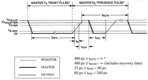
\* In order not to mask interrupt signaling by other devices on the 1-Wire bus,  $t_{RSTL} + t_R$  should always be less than 960  $\mu$ s.
