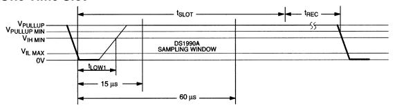
60 μs  $\leq$  t<sub>SLOT</sub> < 120 μs 1 μs  $\leq$  t<sub>LOW1</sub> < 15 μs 1 μs  $\leq$  t<sub>REC</sub> <  $\infty$
