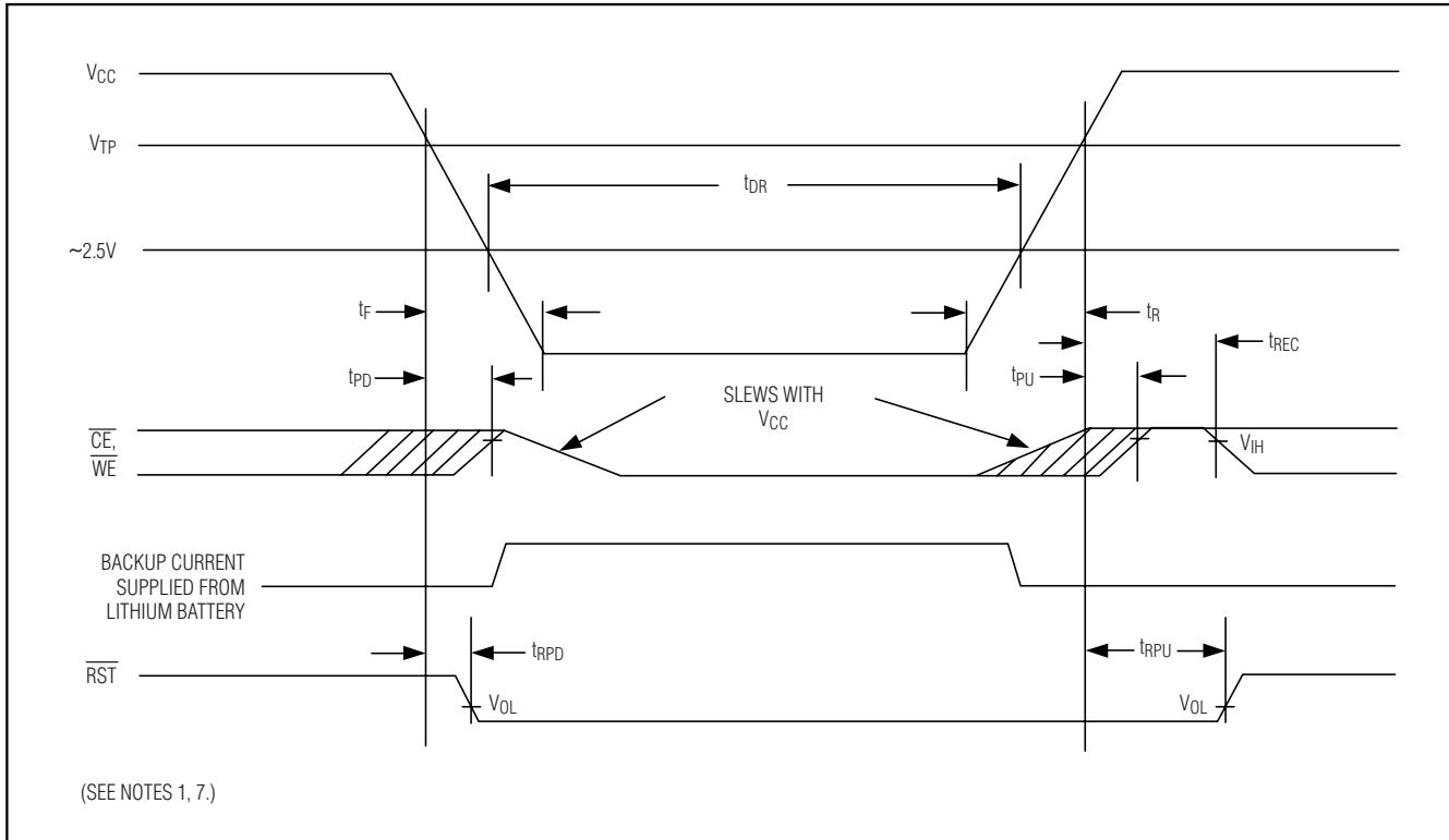
**Note 1:**  $\overline{RST}$  is an open-drain output and cannot source current. An external pullup resistor should be connected to this pin to realize a logic-high level.
