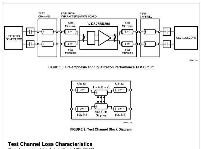
The test channel was fabricated with Polyclad PCL-FR-370-Laminate/PCL-FRP-370 Prepreg materials (Dielectric constant of 3.7 and Loss Tangent of 0.02). The edge coupled differential striplines have the following geometries: Trace Width (W) = 5 mils, Gap (S) = 5 mils, Height (B) = 16 mils.
