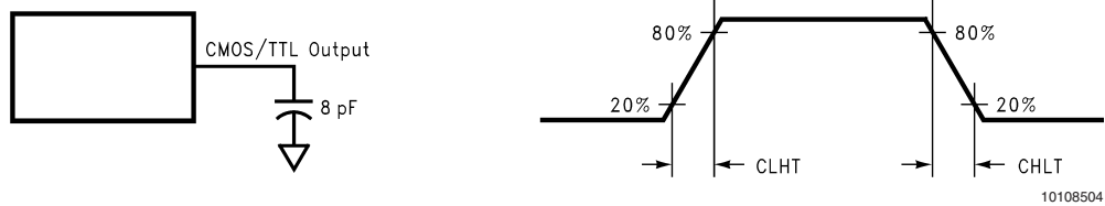
FIGURE 4. DS90CF386/DS90CF366 (Receiver) CMOS/TTL Output Load and Transition Times
