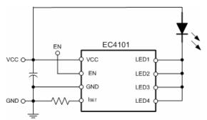
The R<sub>SET</sub> value may be determined as  $R_{SET} = 1.5 * 1200/I_{OUT}$ , k $\Omega$  where 1.5 is a typical I<sub>SET</sub> pin voltage, 1200 is a typical current multiplication ratio, and I<sub>OUT</sub> is a required LED current in mA.
