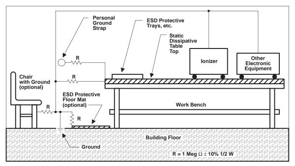
All electrical equipment sitting on the conductive table top must be hard grounded but must be isolated from the static dissipative work surface.
