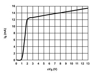
FIGURE 4. SUPPLY CURRENT vs SUPPLY VOLTAGE
