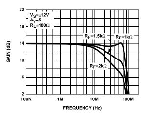
FIGURE 3. DIFFERENTIAL FREQUENCY RESPONSE vs RF
