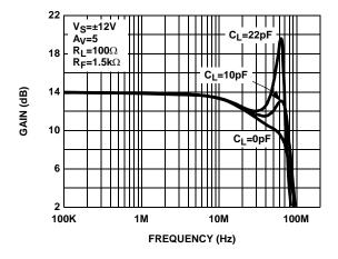
FIGURE 5. DIFFERENTIAL FREQUENCY RESPONSE vs  $C_L$
