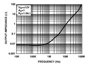
FIGURE 12. OUTPUT IMPEDANCE vs FREQUENCY
