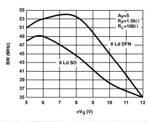
FIGURE 2. DIFFERENTIAL BANDWIDTH vs SUPPLY VOLTAGE
