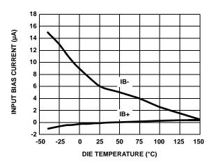
FIGURE 21. INPUT BIAS CURRENT vs TEMPERATURE
