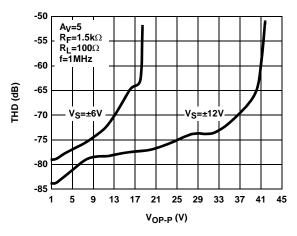
FIGURE 11. DIFFERENTIAL TOTAL HARMONIC DISTORTION
