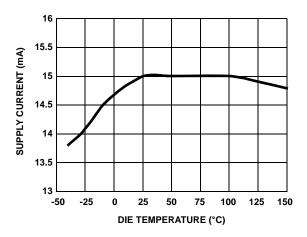
FIGURE 19. SUPPLY CURRENT vs TEMPERATURE
