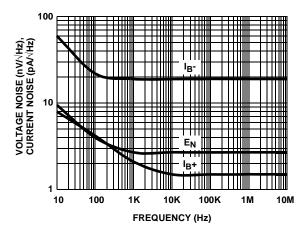
FIGURE 14. VOLTAGE AND CURRENT NOISE vs FREQUENCY
