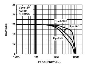
FIGURE 1. DIFFERENTIAL FREQUENCY RESPONSE vs RF
