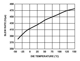
FIGURE 20. SLEW RATE vs TEMPERATURE
