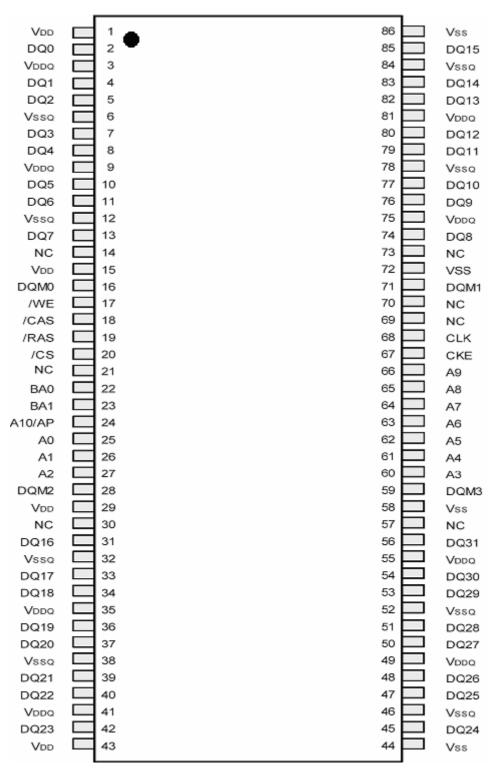
86pin TSOP-II / (400mil × 875mil) / (0.5mm Pin pitch)
