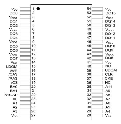
54pin TSOP-II / (400mil × 875mil) / (0.8mm Pin pitch)
