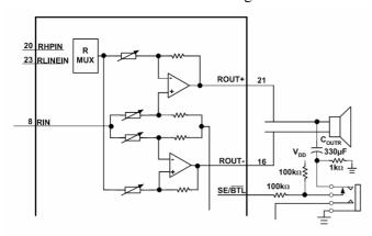
Figure 41. Resistor Divider Network Circuit
