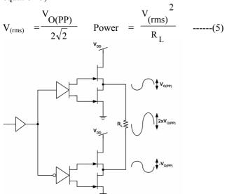
In a typical computer sound channel operating at 5V, bridging raises the power into an 8- $\Omega$  speaker from a singled-ended (SE, ground reference) limit of 250 mW to 1W. In sound power that is a 6-dB improvement—which is loudness that can be heard. In addition to increased power there are frequency response concerns. Consider the single-supply SE configuration shown in Figure 40.
