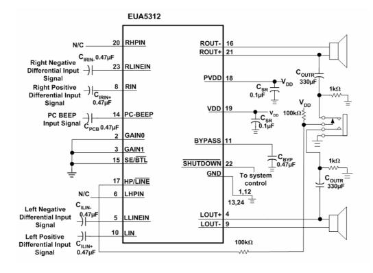
Figure 2. Application circuit using differential input
