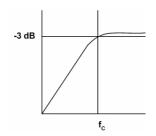
The main disadvantage, from a performance standpoint, is the load impedances are typically small, which drives the low-frequency corner higher, degrading the bass response. Large values of  $C_C$  are required to pass low frequencies into the load. Consider the example where a  $C_C$  of 330 $\mu$ F is chosen and loads vary from 3 $\Omega$ , 4 $\Omega$ , 8 $\Omega$ , 32 $\Omega$ , 10k $\Omega$ , to 47k $\Omega$ . Table 2 summarizes the frequency response characteristics of each configuration.
