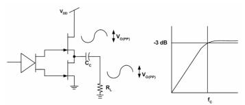
Figure 40. Single-Ended Configuration and Frequency Response
