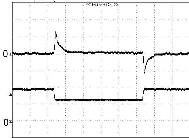
Figure 8: Output voltage response to step-change in load current (75%-50%-75% of I_o , max; di/dt = 0.1A/\mu s ). Load cap: 10\mu F tantalum capacitor and 1\mu F ceramic capacitor. Top Trace: V_{out} (100mV/div, 200us/div), Bottom Trace: I_{out} (2A/div). Scope measurement should be made using a BNC cable (length shorter than 20 inches). Position the load between 51 mm to 76 mm (2 inches to 3 inches) from the module
