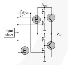
Figure 46. MillerDrive™ Output Architecture
