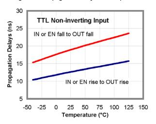
Figure 34. Propagation Delays vs. Temperature
