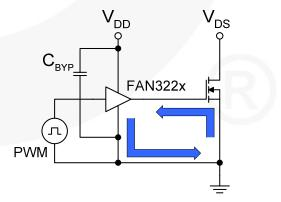
Figure 48. Current Path for MOSFET Turn-off
