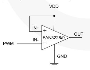
Figure 50. Dual-Input Driver Enabled, Inverting Configuration
