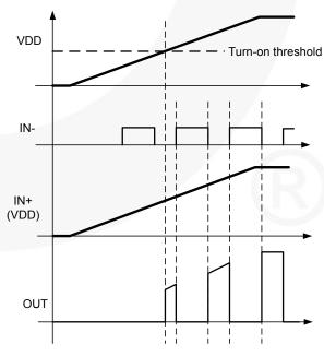
Figure 52. Inverting Start-Up Waveforms
