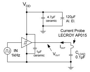
Figure 45. Quasi-Static I<sub>OUT</sub> / V<sub>OUT</sub> Test Circuit
