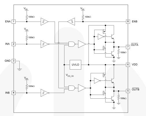
Figure 5. FAN3226 Block Diagram
