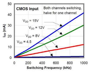
Figure 14. IDD (No-Load) vs. Frequency
