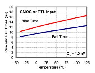
Figure 38. Rise and Fall Times vs. Temperature
