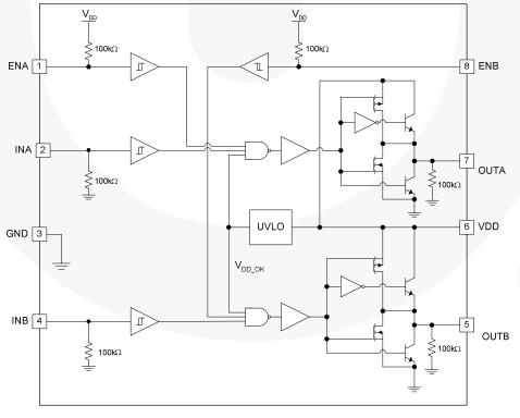
Figure 6. FAN3227 Block Diagram
