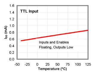
Figure 18. I<sub>DD</sub> (Static) vs. Temperature<sup>(12)</sup>
