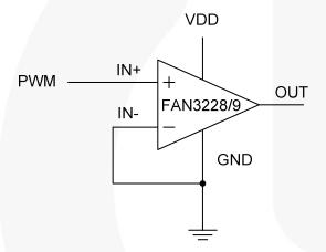
Figure 49. Dual-Input Driver Enabled, Non-Inverting Configuration
