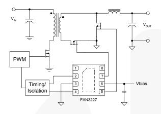
Figure 53. Forward Converter with Synchronous Rectification
