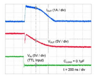
Figure 43. Quasi-Static Source Current with V<sub>DD</sub>=8V
