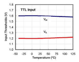
Figure 25. Input Thresholds vs. Temperature
