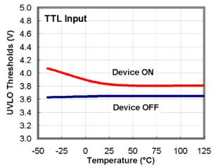
Figure 26. UVLO Thresholds vs. Temperature
