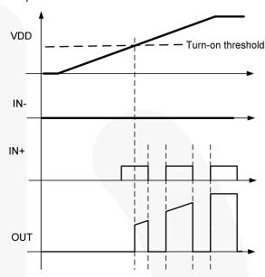
Figure 51. Non-Inverting Start-Up Waveforms
