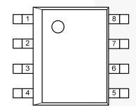
Figure 3. SOIC-8 (Top View)
