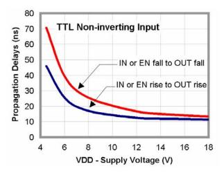
Figure 30. Propagation Delays vs. Supply Voltage
