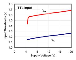
Figure 21. Input Thresholds vs. Supply Voltage
