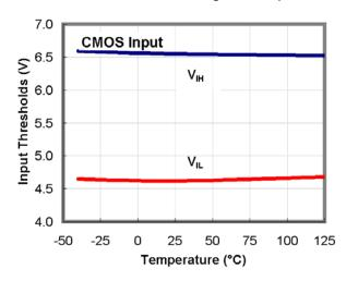
Figure 24. Input Thresholds vs. Temperature
