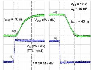
Figure 39. Rise/Fall Waveforms with 1nF Load
