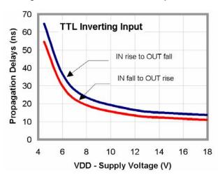
Figure 28. Propagation Delays vs. Supply Voltage
