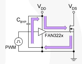
Figure 47. Current Path for MOSFET Turn-on
