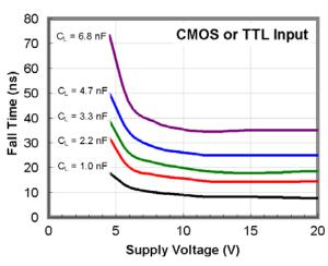
Figure 36. Fall Time vs. Supply Voltage
