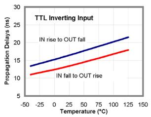
Figure 32. Propagation Delays vs. Temperature
