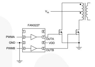
Figure 54. Primary-side Dual Driver in a Push-pull Converter
