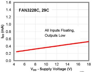
Figure 13. I<sub>DD</sub> (Static) vs. Supply Voltage<sup>(12)</sup>
