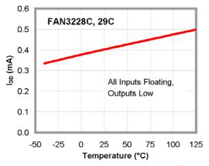
Figure 20. I<sub>DD</sub> (Static) vs. Temperature<sup>(12)</sup>
