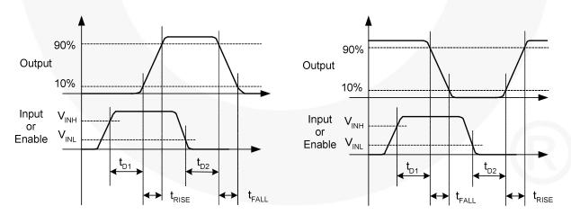
Figure 9. Non-inverting
