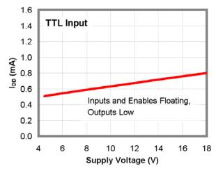
Figure 11. I<sub>DD</sub> (Static) vs. Supply Voltage<sup>(12)</sup>
