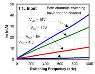
Figure 15. IDD (No-Load) vs. Frequency
