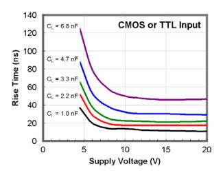
Figure 37. Rise Time vs. Supply Voltage
