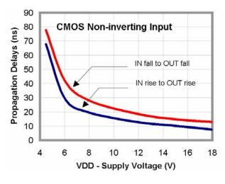
Figure 29. Propagation Delays vs. Supply Voltage
