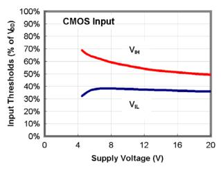
Figure 23. Input Threshold % vs. Supply Voltage
