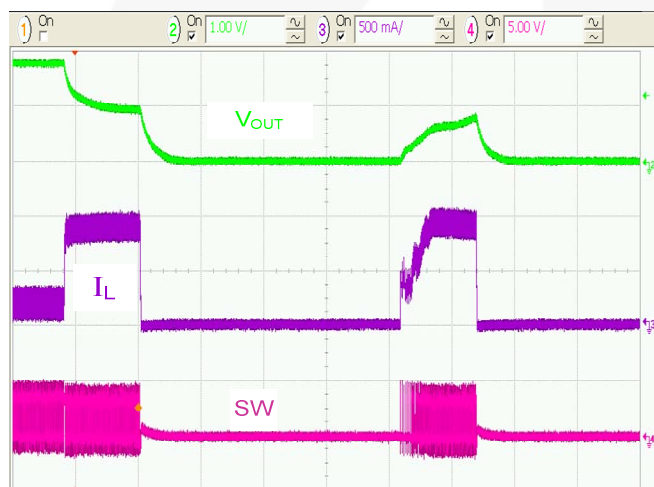
Figure 35. Over-Current Fault Response, R_{LOAD} = 1\Omega , 20\mu s/div.
