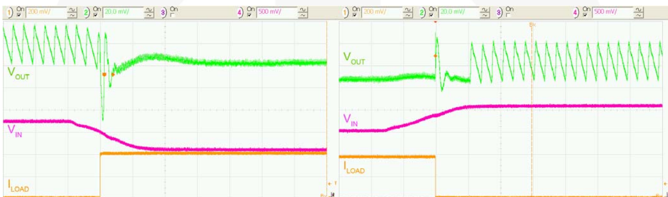
Figure 22. Combined Line/Load Transient 3.3 to 3.9V_{IN} Combined with 400mA to 40mA Load Transient
