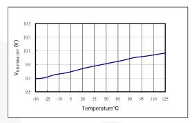
Figure 6. PWM Off Threshold Voltage
