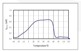
Figure 11. Leakage Current After Startup
