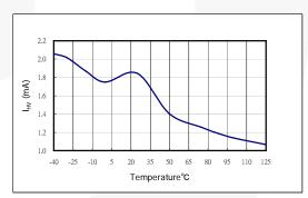
Figure 10. Supply Current Drawn From HV Pin
