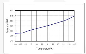
Figure 16. Start Timer (V<sub>FB</sub><V<sub>G</sub>)
