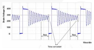
Figure 21. Internal t<sub>TIME-OUT</sub> Initiates New Cycle After Failure to Detect Valley Voltage (with 9µs Delay)
