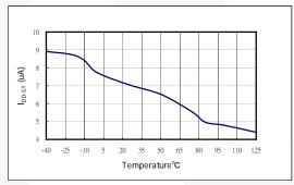
Figure 8. Startup Current
