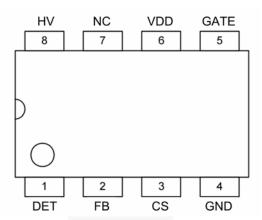
Figure 4. Pin Configuration
