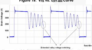
Figure 20. QR Operation in Extended Valley Voltage Detection Mode
