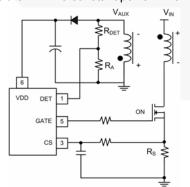
Figure 22. H/L Line Constant Power Limit
