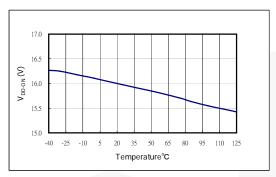
Figure 5. Turn-on Threshold Voltage
