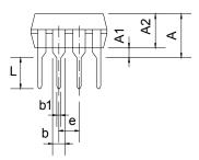
Figure 25. 8-Lead, Dual Inline Package (DIP)
