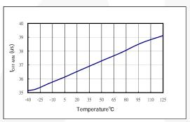
Figure 15. Minimum Off Time (V<sub>FB</sub>=V<sub>G</sub>)
