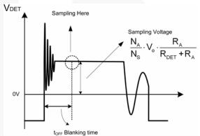
Figure 23. Voltage Sampled After 4µs Blanking Time
