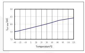
Figure 14. Minimum Off Time (V<sub>FB</sub>>V<sub>N</sub>)
