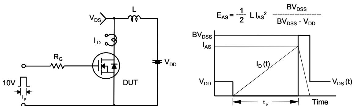
$$E_{AS} = \frac{1}{2} L I_{AS}^2 \frac{BV_{DSS}}{BV_{DSS} - V_{DD}}$$
