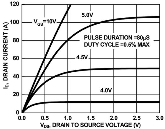
**Figure 8. Saturation Characteristics**
