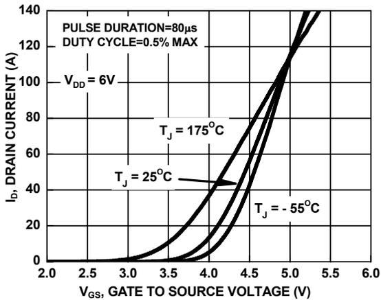
**Figure 7. Transfer Characteristics**
