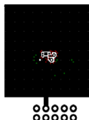
a. 86^\circ\text{C}/\text{W} when mounted on a 1 in 2 pad of 2 oz copper.
