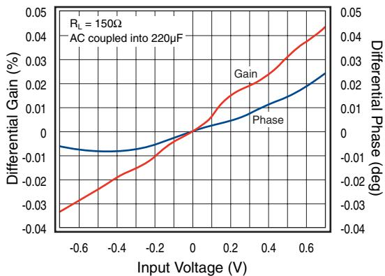
Figure 26. Differential Gain and Phase ( $\pm 5\text{V}$ )
