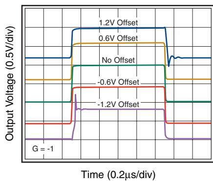
**Figure 22. Large Signal Pulse Response (+3V)**
