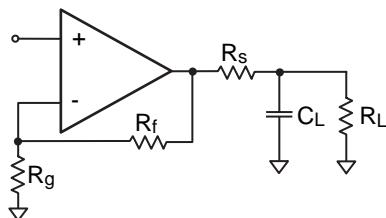
**Figure 27. Typical Topology for Driving Capacitive Loads**
