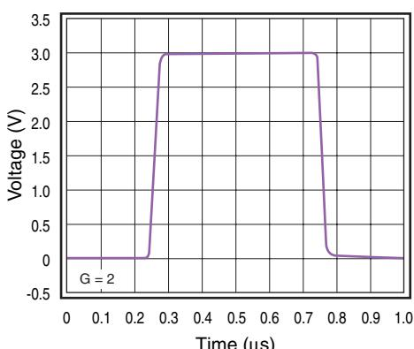
**Figure 24. Large Signal Pulse Response ( $\pm 5\text{V}$ )**
