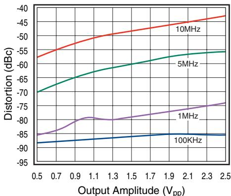
Figure 14. HD3 vs.  $V_O$  (+5V)
