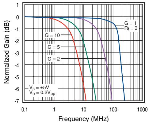
Figure 2. Inverting Freq. Response ( $\pm 5\text{V}$ )
