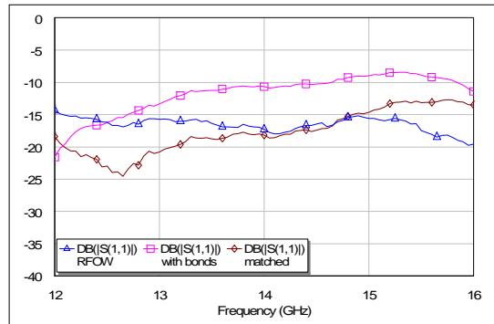
Once bonded the return losses are still at a reasonable level. They can be improved with simple compensation networks. The figures also show the effect of this bondwire compensation network (brown diamonds). The networks are shown at the end of this section.
