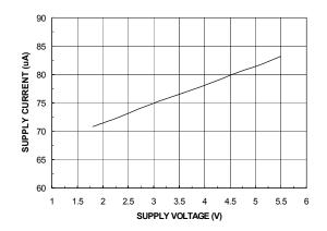
Figure 1. Quiescent Current vs. Input Voltage
