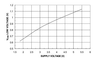
Figure 4.  $V_{ONB}$  Low Voltage vs. Input Voltage
