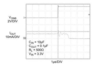
Figure 12.  $T_{OFF}$  Response
