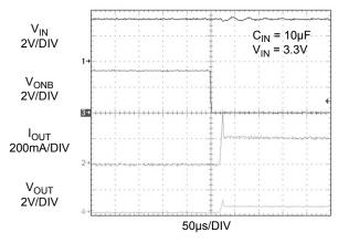
Figure 15. Current Limit Response Time (Output is loaded by  $2.2\Omega$ ,  $C_{OUT}$  =  $0.1\mu F$ )
