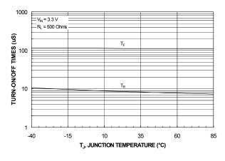
Figure 10.  $T_{\mbox{\scriptsize RISE}}$  /  $T_{\mbox{\scriptsize FALL}}$  vs. Temperature
