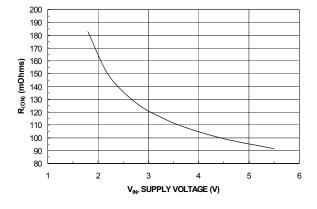
Figure 5.  $R_{(ON)}$  vs.  $V_{IN}$
