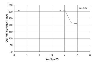
Figure 7. Current Limit vs. Output Voltage
