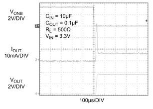
Figure 11.  $T_{ON}$  Response
