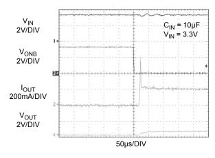
Figure 16. Current Limit Response Time (Output is loaded by 2.2 $\Omega$ ,  $C_{OUT}$  = 10 $\mu$ F)
