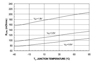
Figure 6.  $R_{(ON)}$  vs. Temperature
