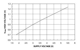
Figure 3.  $V_{ONB}$  High Voltage vs. Input Voltage
