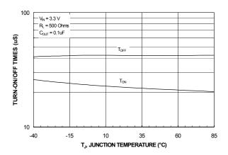
Figure 9.  $T_{ON}$  /  $T_{OFF}$  vs. Temperature
