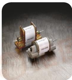
An open frame RF reed relay with 8kV isolation and 6A (at 30MHz) carry current, the FRD12000 series has been used in many HF radio system specifications over the years, with applications in commercial maritime (GMDSS) equipment and military HF radio units worldwide. The use of vacuum reed switches with rhodium contacts offers high isolation voltages, low contact resistance and long operating lifetime.
