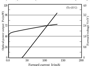
Optical power output - Forward current [Pulse]
