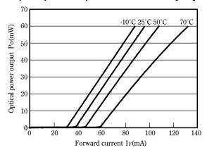
Case temperature dependence of threshold current [CW]
