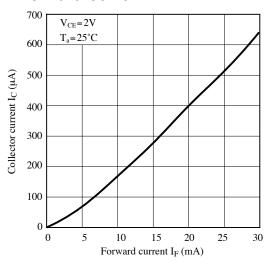
Fig.6 Relative Collector Current vs.
