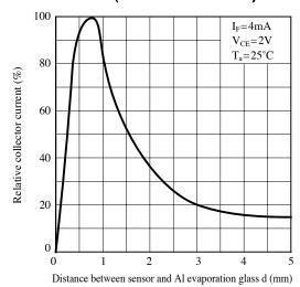
Fig.11 Detecting Position Characteristics (1)
