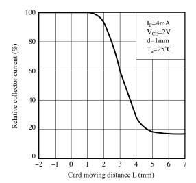
Fig.12 Detecting Position Characteristics (2)
