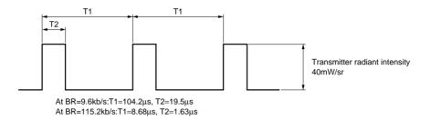
Fig.4 Output Waveform Specification (Receiver side)
