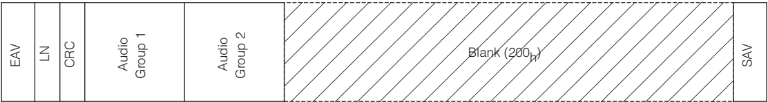
Video Signal before GS1503 (with existing Audio Data Packets)
