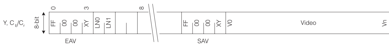
Fig. 12 Video Input Format 8-bit with TRS and Line Numbers
