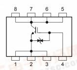
These devices are MOS type. Users should follow proper ESD handling procedures. perating condition of turn-off dv/dt should be lower than 400 V/µs.
