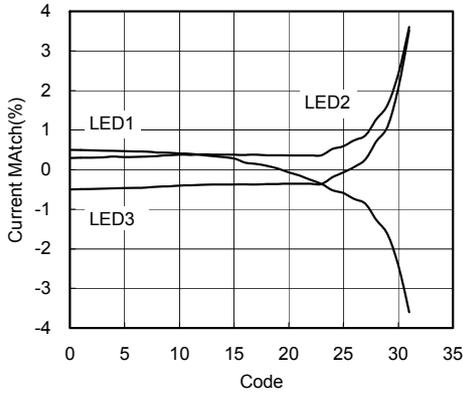
Current Match vs.  $V_{LED}$
