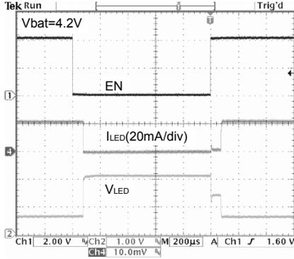
Linear Dimming Waveform I
