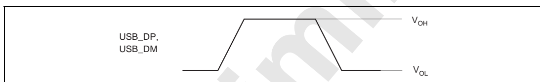
Figure 33.66 Output ( V_{OH} , V_{OL} )
