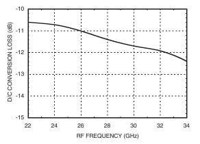
Note 1: Single side band measurement without  $90^{\rm o}$  hybrid, and second IF port terminated.
