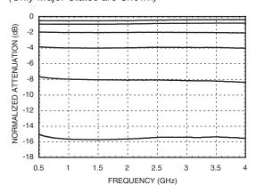
Bit Error vs. Attenuation State
