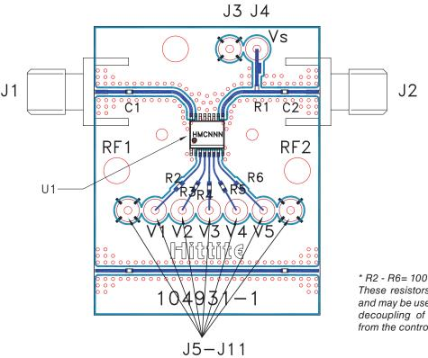
\* R2 - R6= 100 Ohm. These resistors are optional and may be used to enhance decoupling of the RF path from the control inputs.
