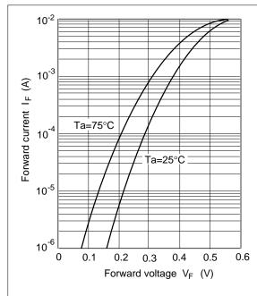
Fig.1 Forward current Vs. Forward voltage
