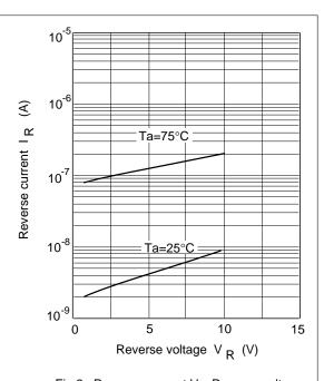
Fig.2 Reverse current Vs. Reverse voltage
