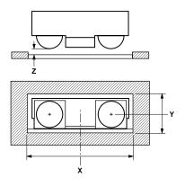
X is the width of the window, Y is the height of the window, and Z is the distance from the HSDL-3200 to the back of the window.
