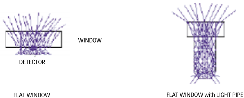
Figure 12. Recommended window design.
