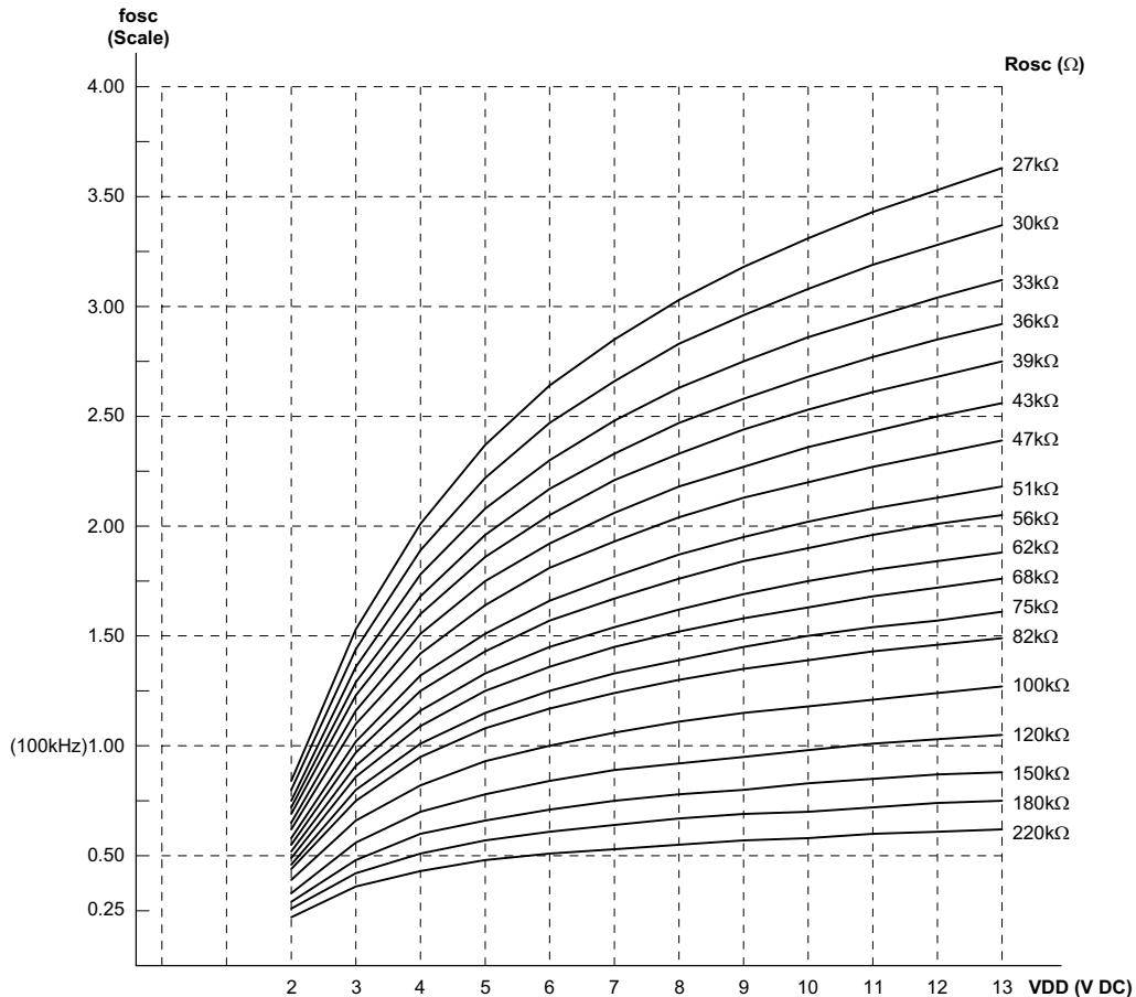
Note: The recommended oscillator frequency is  $f_{OSCD}$  (decoder)  $\cong 50 f_{OSCE}$  (HT12E encoder)
