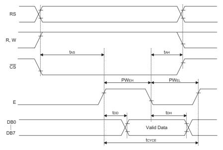
Note: The input signal rising time and falling time  $(t_f, t_r)$  is specified at 15ns or less. All timing is specified using 20% and 80% of V<sub>DD</sub> as the reference. PW<sub>EH</sub> is specified as the overlap between  $\overline{CS}$  being L and E.
