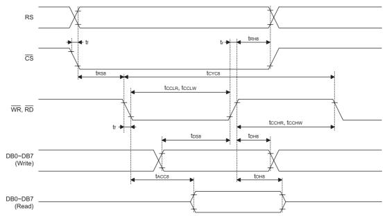
Note: The input signal rising time and falling time  $(t_{f},\,t_{r})$  is specified at 15ns or less.
