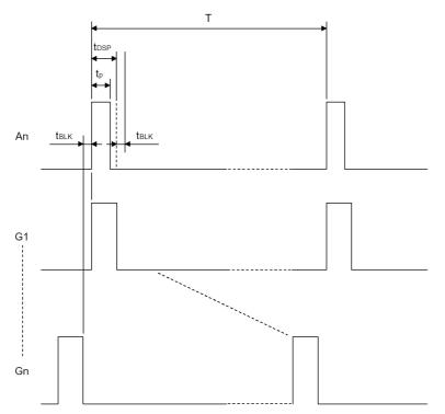
Note: "n" means number of grid, T=nx (t<sub>DSP</sub>+t<sub>BLK</sub>)
