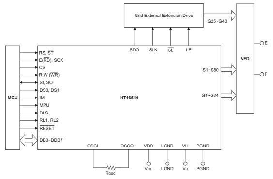
Note:  $R_{OSC}$ =56k $\Omega$  for oscillator resistor
