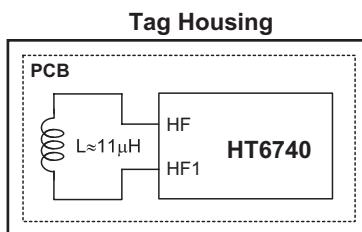
Note: The value of the antenna inductance is  $11\mu H$ , however the optimum value will be changed slightly due to the variation of the internal resonance capacitor (10pF typically) during process.
