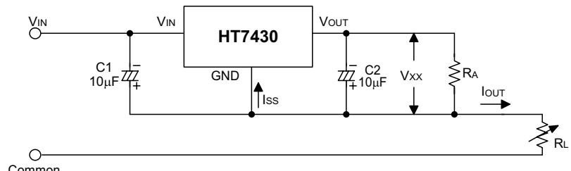
$$I_{OUT} = \frac{V_{xx}}{R_A} + I_{ss}$$
