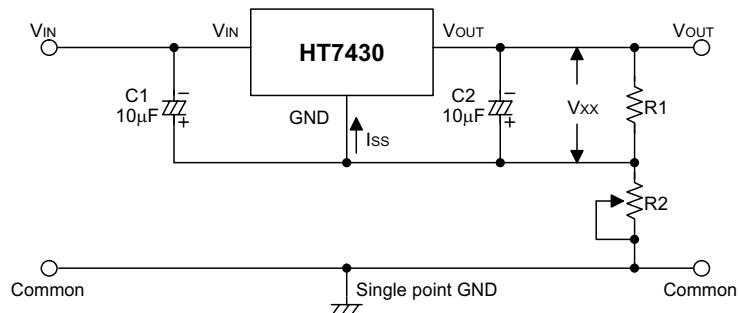
$$V_{OUT} = V_{xx} \left( 1 + \frac{R_2}{R_1} \right) + I_{ss} R_1$$
