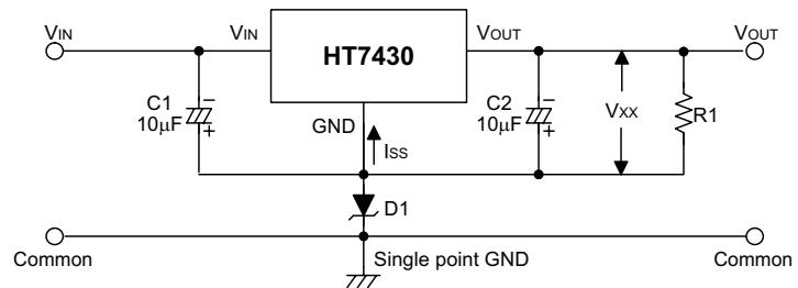
$$V_{OUT} = V_{xx} + V_{D1}$$
