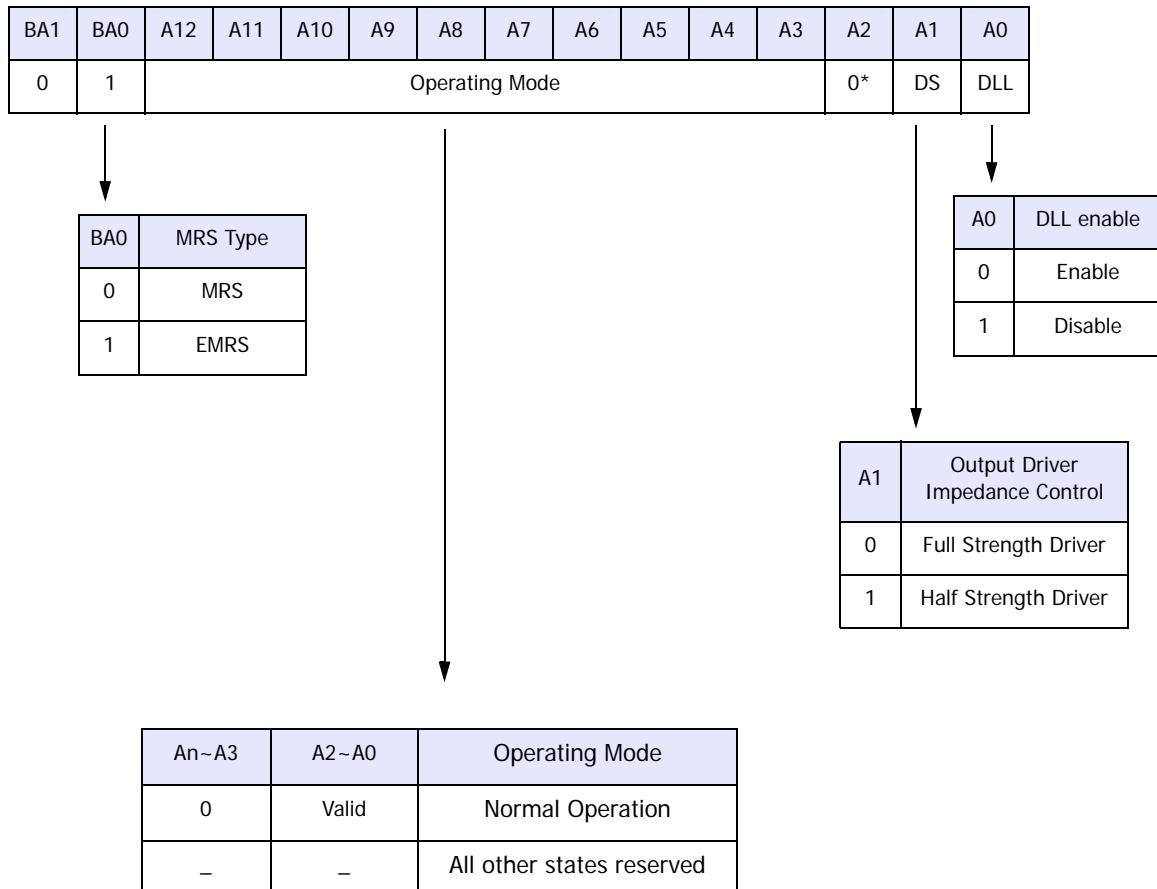
\* This part do not support/QFC function, A2 must be programmed to Zero.
