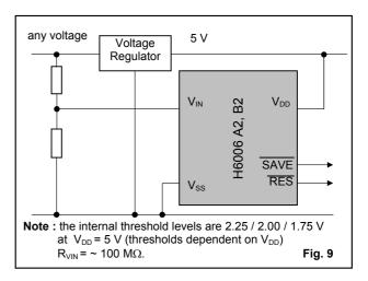
**Version A3, B3:** for monitoring of regulated voltage, where no unregulated voltage is available (the tolerance is  $\pm 10$  %, see Table 4. For tighter tolerances, trimming can be used, see Fig. 10).
