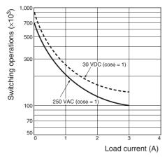
Reference: A maximum current of 0.15 A can be switched at 125 VDC ( $\cos\phi = 1$ ) and a maximum current of 0.1 A can be switched if L/R is 7 ms. In both cases, a life of 100,000 operations can be expected. The minimum applicable load is 10 mA at 5 VDC (failure level: P).
