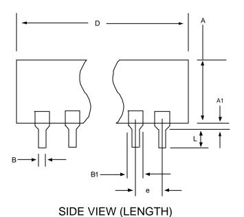
Package Dimensions for 40 Lead PDIP (600 mil.)
