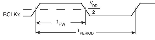
$$odc = \frac{t_{PW}}{t_{PERIOD}} \times 100\%$$
