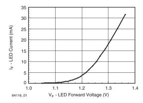
Fig. 5 - LED Forward Current vs. Forward Voltage
