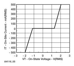
Fig. 9 - On-State Terminal Voltage vs. Terminal Current
