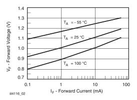
Fig. 6 - Forward Voltage vs. Forward Current
