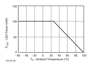
Fig. 8 - Maximum LED Power Dissipation
