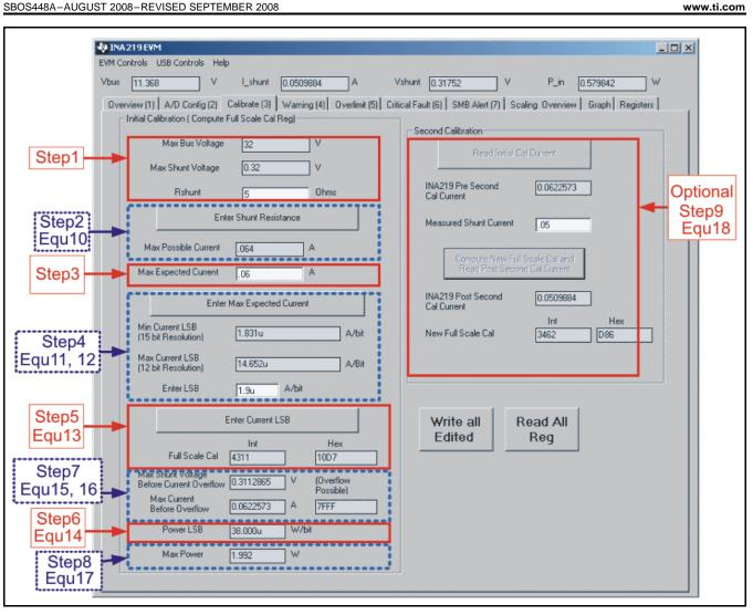
Figure 22. Calibration Software Automatically Computes Calibration Steps 1-9
