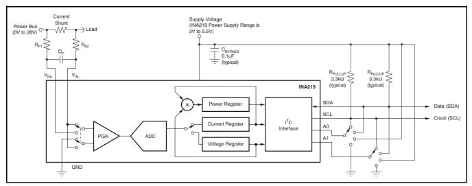
Figure 13. Typical Application Circuit
