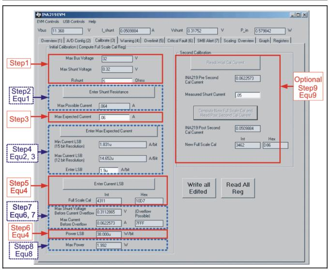
Figure 21. INA219 Calibration Sofware Automatically Computes Calibration Steps 1-9
