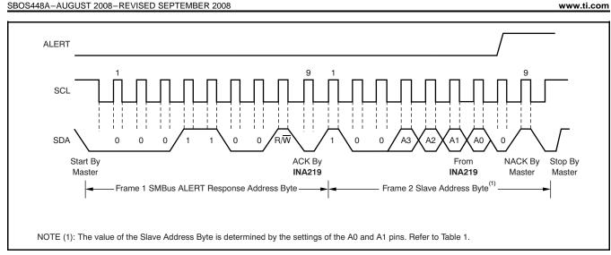
Figure 16. Timing Diagram for SMBus ALERT
