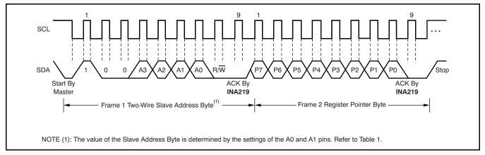
Figure 17. Typical Register Pointer Set
