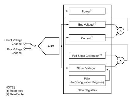
Figure 12. INA219 Register Block Diagram
