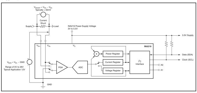
Figure 19. INA219 Configured for Shunt and Bus Voltage Measurement
