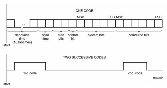
Where: debounce time + scan time = 18 bit-times repetition time = 4 ' 16 bit-times
